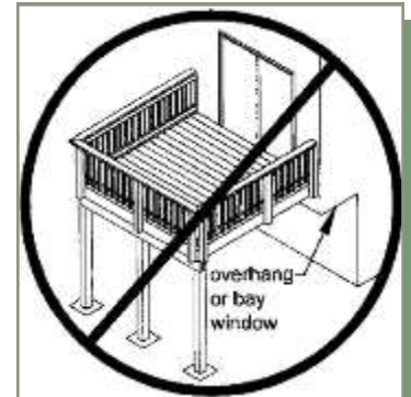
Figure 18: No Attachment to House Overhang
